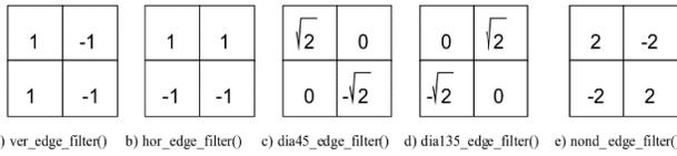
Fig. 7: Filters for edge detection
