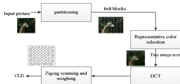
Fig. 2: The CLD extraction process block diagram
